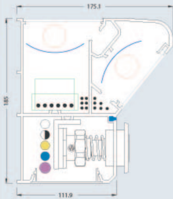
Profile "ELISA" for normal hospital care and critical area for horizontal and suspended mounted
